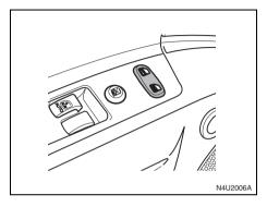
If your vehicle has this feature you can unlock or lock the doors on your vehicle using the driver's door lock switch. Push down the front part of the switch to unlock the doors. Push down the back part of the switch to lock the doors.
